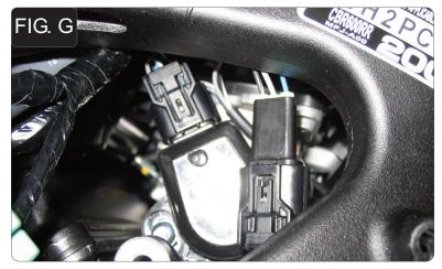
Plug the BLACK connectors from the PCV in-line of the stock TPS and wiring harness (Fig. G).
