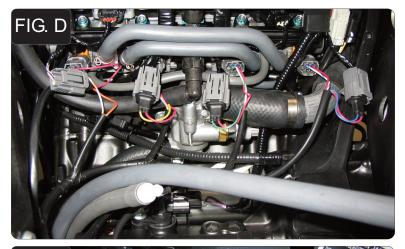
9 Plug the PCIII wiring harness in-line of the stock injectors and stock wiring harness (Fig. D).
