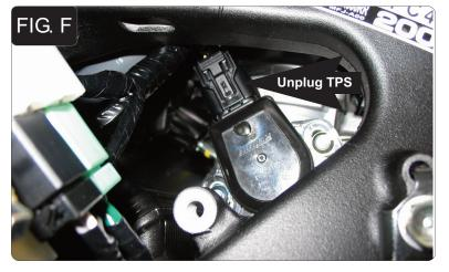
11 Unplug the stock wiring harness from the Throttle Position Sensor (Fig. F).
