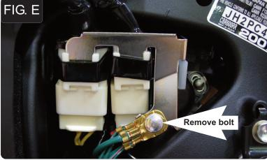
Remove the bolt that holds the ground wires and bracket for the alternator connectors to the frame on the left hand side of the bike.
