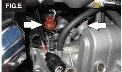
10 Unplug the stock wiring harness from each one of the injectors (Fig. E).
