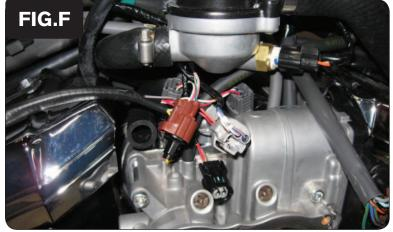
11 Plug the PCV harness in-line of the stock wiring harness and each injector (Fig. F)
