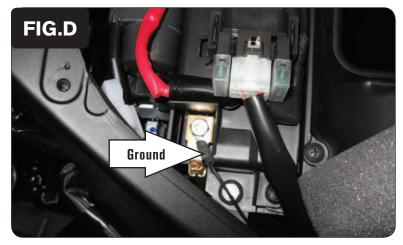
7 Attach the ground wire of the PCV to the negative side of the battery (Fig. D).
