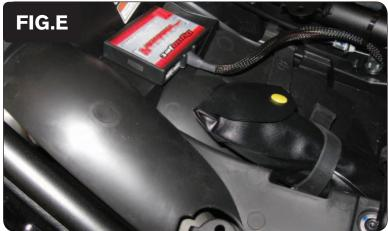
8 Secure the PCV unit in the tail section using the supplied velcro (Fig. E).
