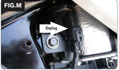
19 Unplug the O2 sensor from the rear exhaust pipe (Fig. M). This connection is located under the right hand side cover.
