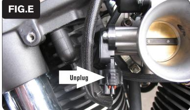
9 Locate the stock Thottle Position Sensor connector. This connector is on the right side of the bike to the rear of the throttle body.
