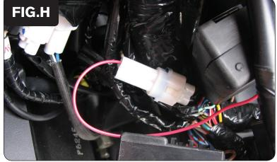
14 Plug the RED wire from the PCV into the stock wiring harness (Fig. H)
