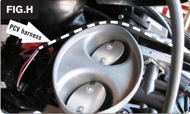
11 Loosen the clamp that holds the intake duct to the throttle body. Lift up on the intake duct so the PCV harness can be routed underneath this duct and in front of the throttle body (Fig. H).
