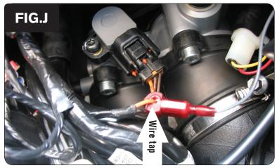
Locate the Throttle Position Sensor wiring harness on the left hand side of the throttle bodies.
