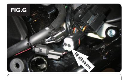
12 Locate the stock O2 sensor connection.
