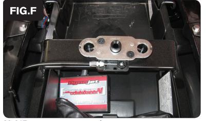
Install the PCV in the tail section using the supplied velcro. Make sure to clean both surfaces with the alcohol swab before attaching (Fig. F).
