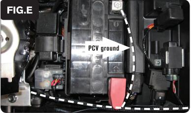
Attach the ground wire from the PCV to the negative side of the battery (Fig. E).
