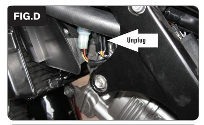
5 Plug the PCV in-line of the stock wiring harness and throttle body harness (Fig. D).
