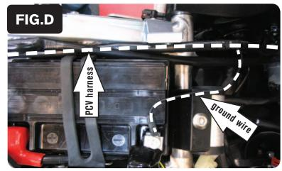
9 Attach the ground wire from the PCV to the negative side of the battery as shown in Figure D.
