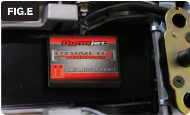
10 Using the supplied velcro, secure the PCV in the tail section as shown in Figure E.
