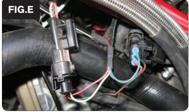
Plug the connectors from the PCV with the GREEN wires in-line of the stock ignition coil and wiring harness (Fig. E).
