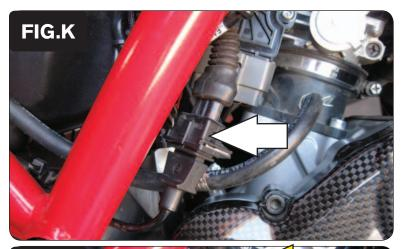
Unplug the crank position sensor connector on the right side of the motorcycle (Fig. K).
