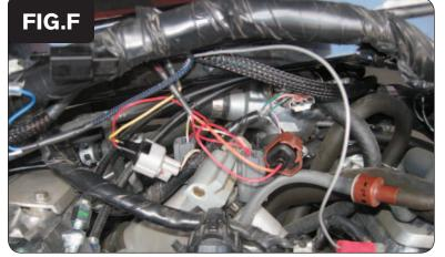
10 Route the remainder of the PCV wiring harness towards the right hand side of the bike, through the frame, under the fuel tank, and towards the throttle bodies while following the stock wiring harness on the right hand side of the frame as closely as possible.
